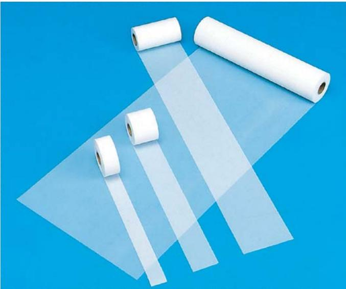
The NAFLON PTFE tape is made by cutting a molded cylindrical PTFE block into a thin tape of the required thickness. It offers a combination of PTFE's excellent characteristics including electrical properties, non-adherent property and low coefficient of friction.
