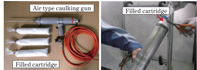
Figure 3 Air type caulking gun and cartridge loading
